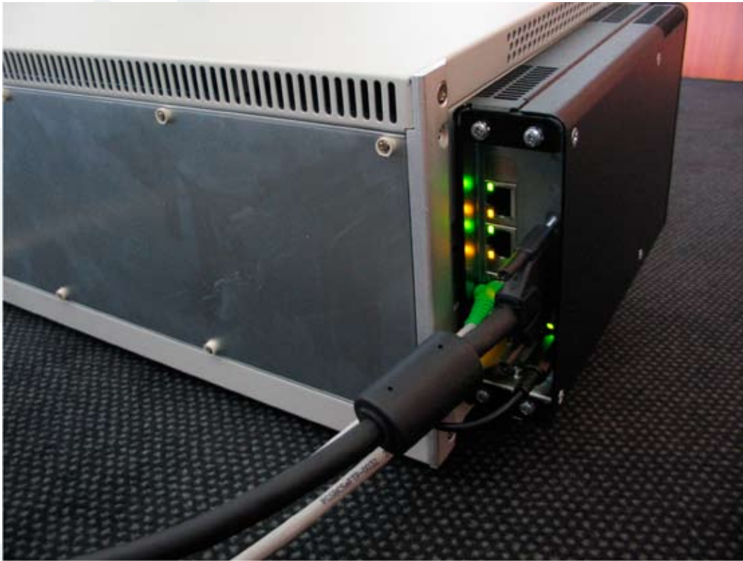
Figure 3 - Expansion box rear view, connection to PXI Interface and PCMCIA card
