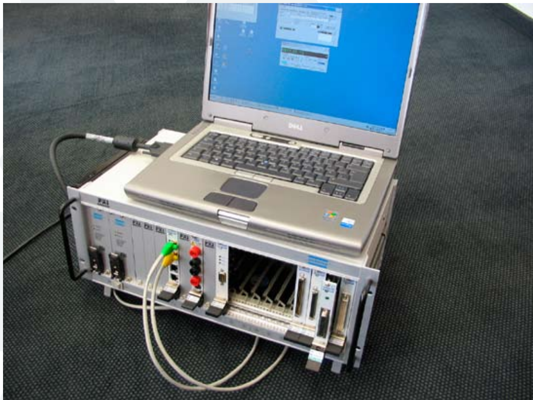
Figure 4 - Notebook connected to chassis via PCI Expansion Box
