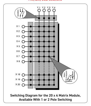
A **shielded 24 pole analogue bus** is provided on the System 20 Analogue Backplane so constructing large matrices is very straight forward, no time consuming daisy-chained wiring harnesses etc.
