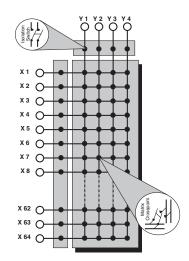
Switching Diagram for the 20-534A 64 x 4 Matrix, Available as Single or Double Pole
