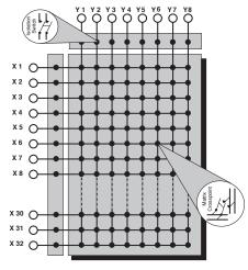
Switching Diagram for the 20-535A 32 x 8 Matrix, Available as Single or Double Pole
