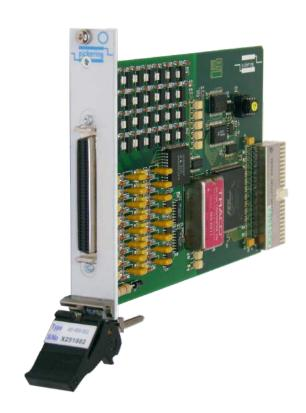
The 40-490/491 module is designed for applications requiring optically isolated digital I/O, typically in industrial automation. The module features 32 digital outputs and 16 digital inputs that can be programmed by word or individual bit.
