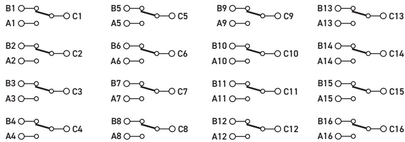
40/42-158-003/103 Power Relay Module Switching Architecture - 16 x SPDT
