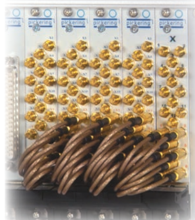
Optional Y-axis loop-thru allows easy expansion. Shown here is a 60x8 RF matrix with over 200 MHz bandwidth.
