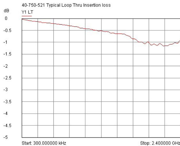
40-750-521 RF Matrix Typical Insertion Loss Plot Using Loop Thru
