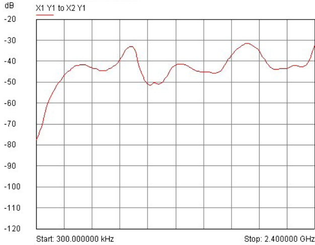
40-750-521 RF Matrix Typical Crosstalk Plot
