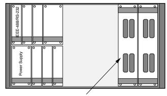
Try To Keep High Voltage Modules Away From Sensitive Switching Modules
