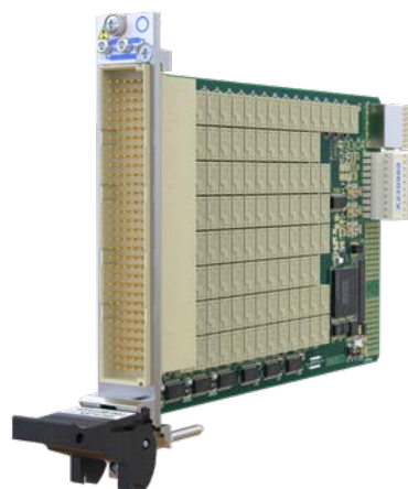
42-612B-002 Very High Density Versatile Multiplexer Module in PXle Format
