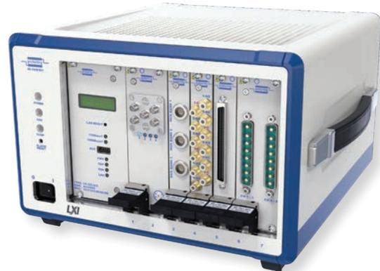
The 60-102B is compliant with the LXI Standard 1.4 and supports Pickering Interfaces 3U PXI switching and simulation modules as though they are an LXI compliant device, complete with a driverless soft front panel. The 60-102B supports up to seven 3U modules and is equivalent to an 8 slot PXI chassis.
