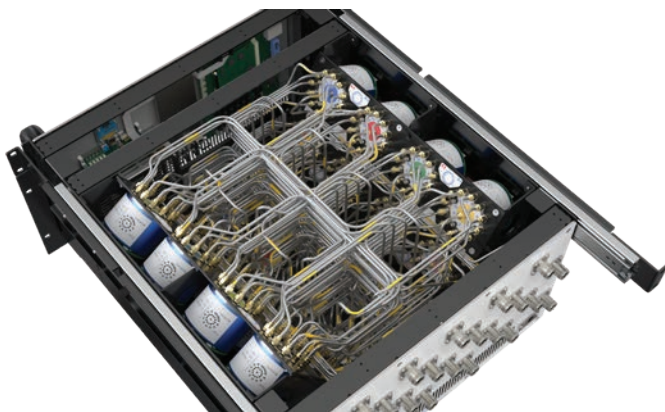
60-891-007 12x12 Microwave Matrix with top cover removed showing internal cabling
