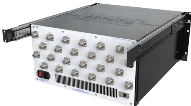
60-891-007 12x12 Microwave Matrix rear view showing signal connectors
