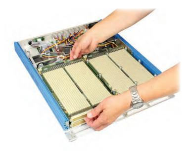
The mother card can be removed by lifting it upwards to disengaging it from the connectors linking it to the card below.
