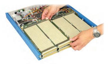
Locate the mother card onto the fixing pillars and press down firmly to fully engage the two connectors in the same way as the upper right mother card.
