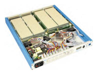
Remove the cover by sliding it towards the rear of the unit.
