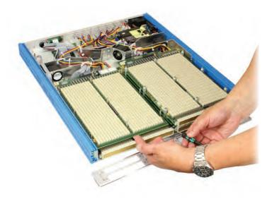
Removal of the daughter card requires it to be disengaged from the connectors linking it to the lower mother board. These can be tight and careful levering with a screwdriver can help.
