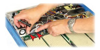
To remove the data cables, push the black retaining levers away from each other to eject the connector.
