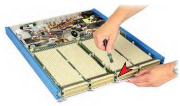
Next remove the screw securing the earth wires to the front panel.
