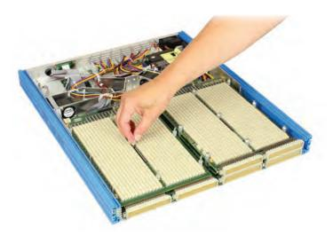
• Fit the upper left mother card by first fitting nine spacers to the fixing pillars.
