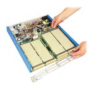
Once the screws and spacers have been removed, the mother card can be removed by lifting it upwards to disengaging it from the connectors linking it to the card below.
