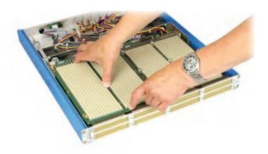
Locate the daughter card onto the fixing pillars and press down firmly to fully engage the connectors linking it to the mother card below.
