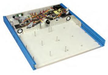
With the matrix cards removed from the chassis, the required repairs can be carried out before re-assembly.
