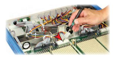
Before removal of the lower mother cards, the four power cables and four data cables have to be disconnected. As there is limited space behind the boards, the power connectors can be removed by carefully levering them free with a screwdriver.
