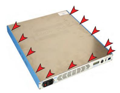
Remove the twelve fixing screws securing the top cover to the chassis.
