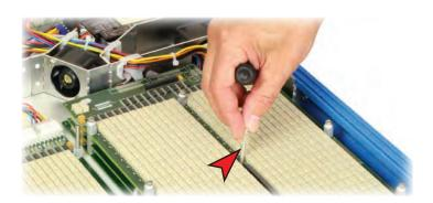
When removing the card fixing screws, sometimes the whole pillar becomes detached. This is not a problem, but greater care will be required when the cards and spacers are re-fitted.
