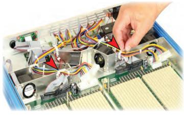
Card removal is made easier if the cables are positioned out of the way. To do this, first release the two cable clamps.
