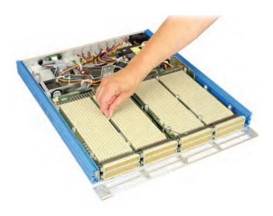
With the front panel separated from the chassis, remove the nine spacers from the top of the upper left matrix mother card.
