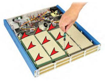
To remove the upper left matrix daughter card, first remove the nine fixing screws securing it to the circuit boards below.
